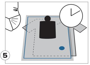
Start the timer and observe the test frequently during 40 minutes. Record the time of positive reaction (distinct area of diffuse blue color).
